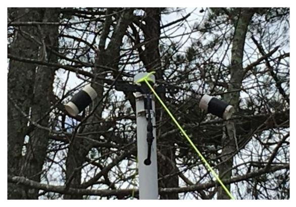
NVIS with only 80 Meter Coils
