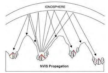
not bounce off the F layer at these sharp angles and just goes out into space. Remember the Maximum Useable Frequency (MUF? For amateur radio operators, we're looking at 40 and 80 meters primarily for NVIS use.
