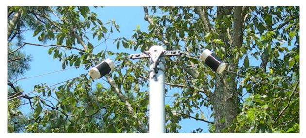
The kit is held onto the PVC conduit using two stainless hose clamps and I topped off the conduit with a white PVC 2 inch cap to keep rain from entering.
