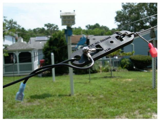
The grey AWG 16 wire is the 32 foot radial and a ¼ inch stab connector is crimped on the end. A stainless steel 5 mm stud is installed to terminate a jumper (with mating ¼ inch stab) and the 12 foot radial for 60 meters (black AWG 14). The other end of the black 12 foot radial is terminated in another insulator and is guyed to a ground stake.
