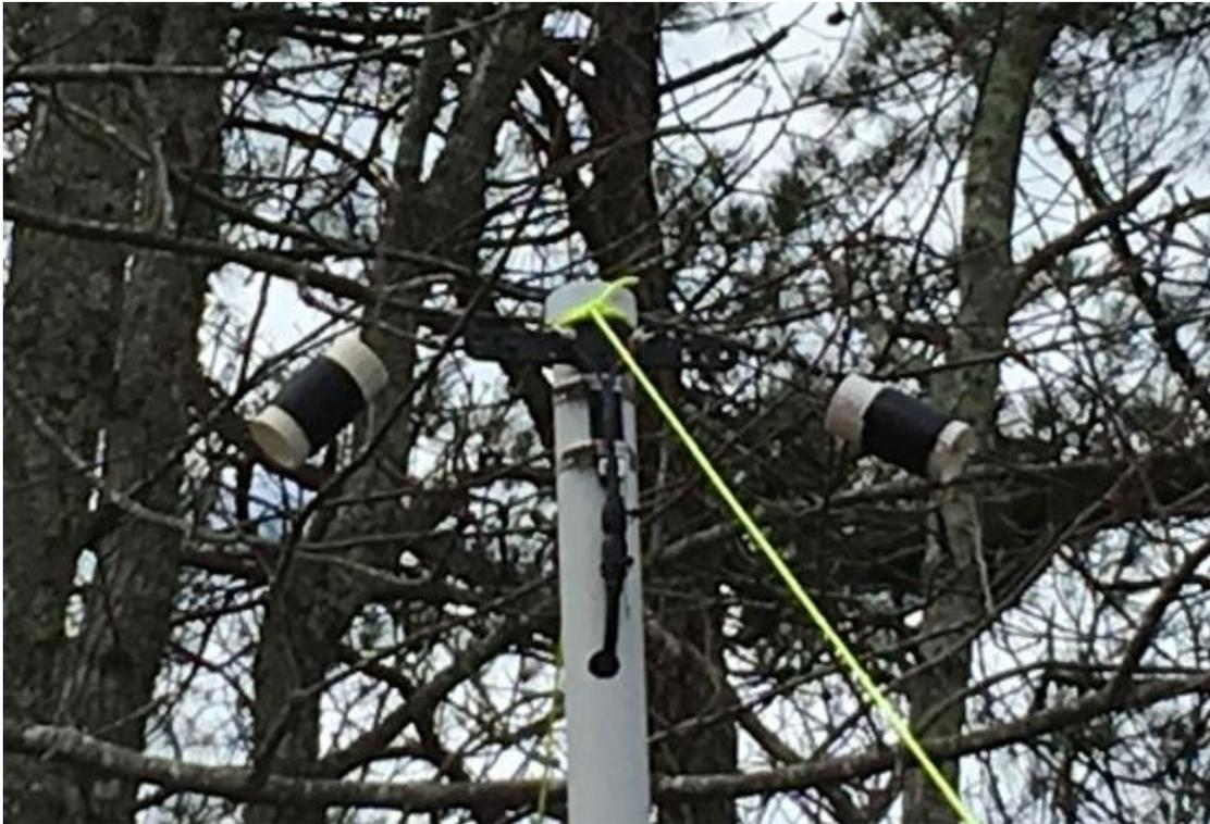
NVIS with only 80 Meter Coils
